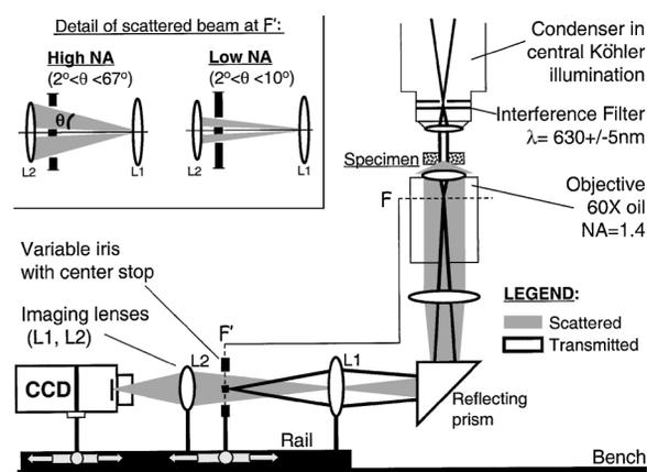
Fig. 1. OSI setup. F, objective's back focal plane; F and F' are conjugate Fourier planes. The scattered light (gray beam) is used to image the specimen on the CCD, and the transmitted light (black ray traces) is blocked at F'. The inset shows the scattered angles passed at the high- and low-NA settings.
