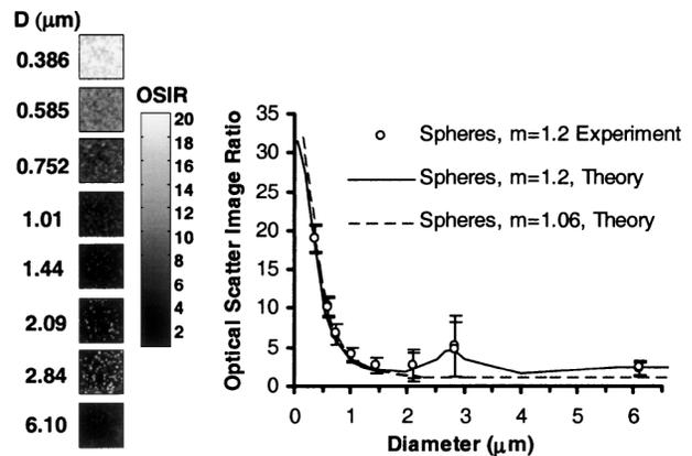
Fig. 2. OSI images and measurement of the OSIR in aqueous suspensions of polystyrene spheres. Experimental data (open circles, refractive-index ratio  $m = 1.2$ ), theoretical predictions (solid curve,  $m = 1.2$ ; dashed curve,  $m = 1.06$ ). The data in the graph are the mean plus or minus the standard deviation of pixel values in the images shown on the left.
